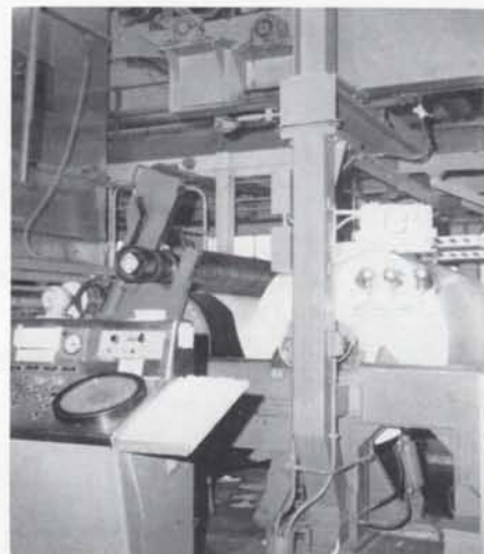
Steel reel is moved into place at wind-up end of coater to start new roll.
