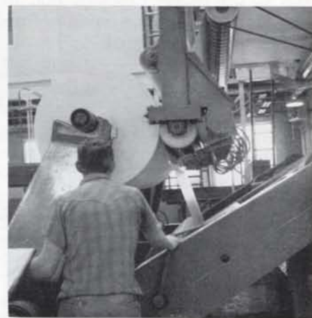
Employee controls flying paster operation.
